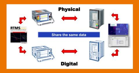
With this concept, the number of potential errors, especially human errors, is minimized, as the transition from virtual tests to physical tests is based on file transfers.
